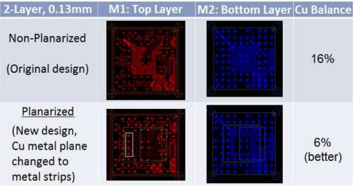
Fig. 10. Proposed substrate design with metal strip design
