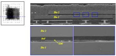
Cross-section photo of SN1 shows total gap between DAF (of Die2) and Die1 interface. Mold compound (EMC) is evident between this gap.
