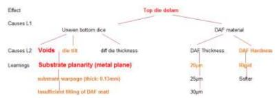
Fig. 5. Fault-tree analysis
