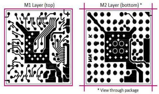
Fig. 2. Substrate design layout top and bottom view
