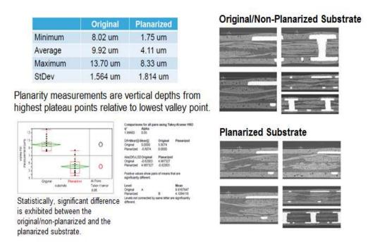
Fig. 7. Comparison between non-planarized and planarized substrate
