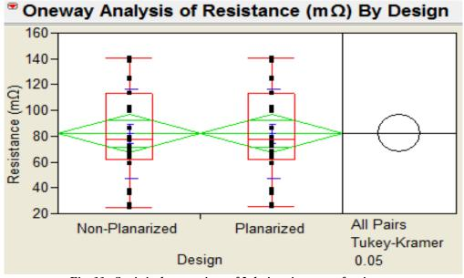
Fig. 11. Statistical comparison of 2 designs in terms of resistance
