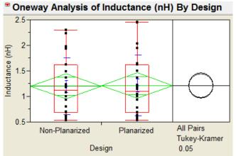
Fig. 12. Statistical comparison of 2 designs in terms of inductance
